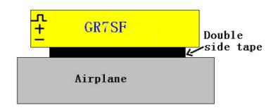
Ensure the axis direction is out of four kind types description below. Fixed GR7SF reference the information mentioned in axis description pictures on receiver's box.
